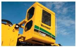
**ELEVATING ENCLOSED CAB.** The elevating cab allows superior visibility and added comfort with the air ride seat. The sealed cab has self-contained heating and air conditioning with sound attenuating foam. It is also a rollover module (ROM).
